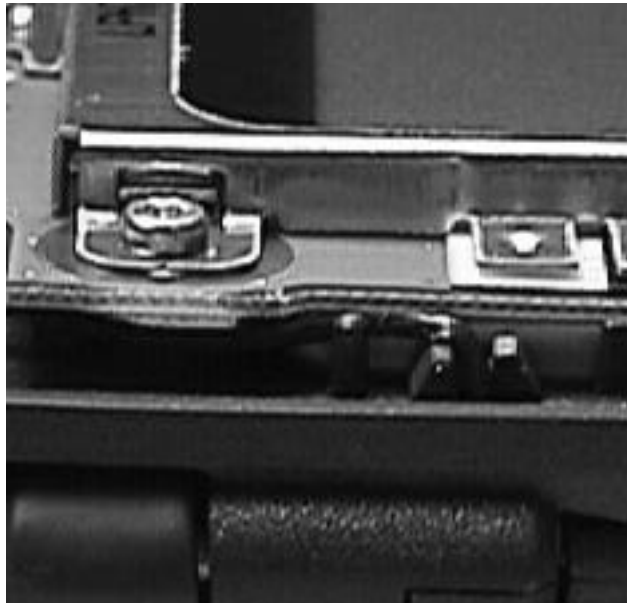
Figure1. Correct way to assemble the coaxial cable in the lid part.
